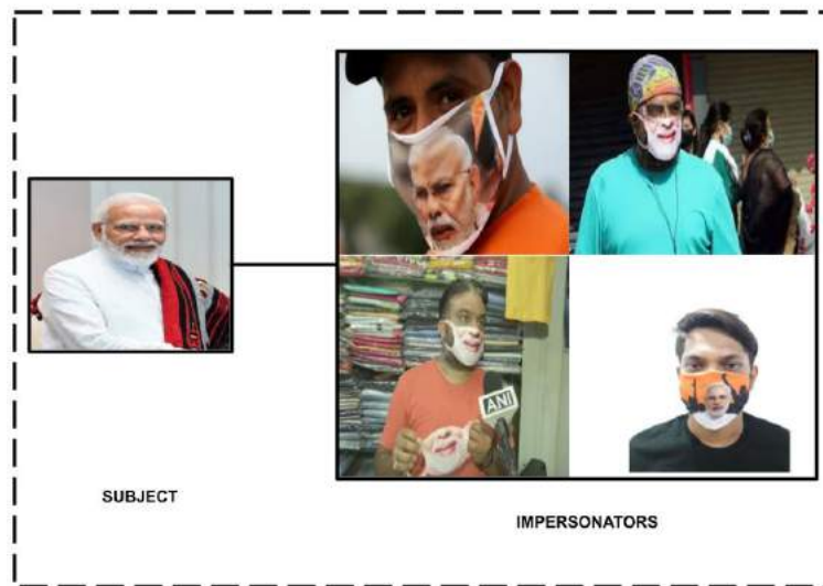
Figure 2.4: Image showing how face print can pose a challenge for face detection and recognition
